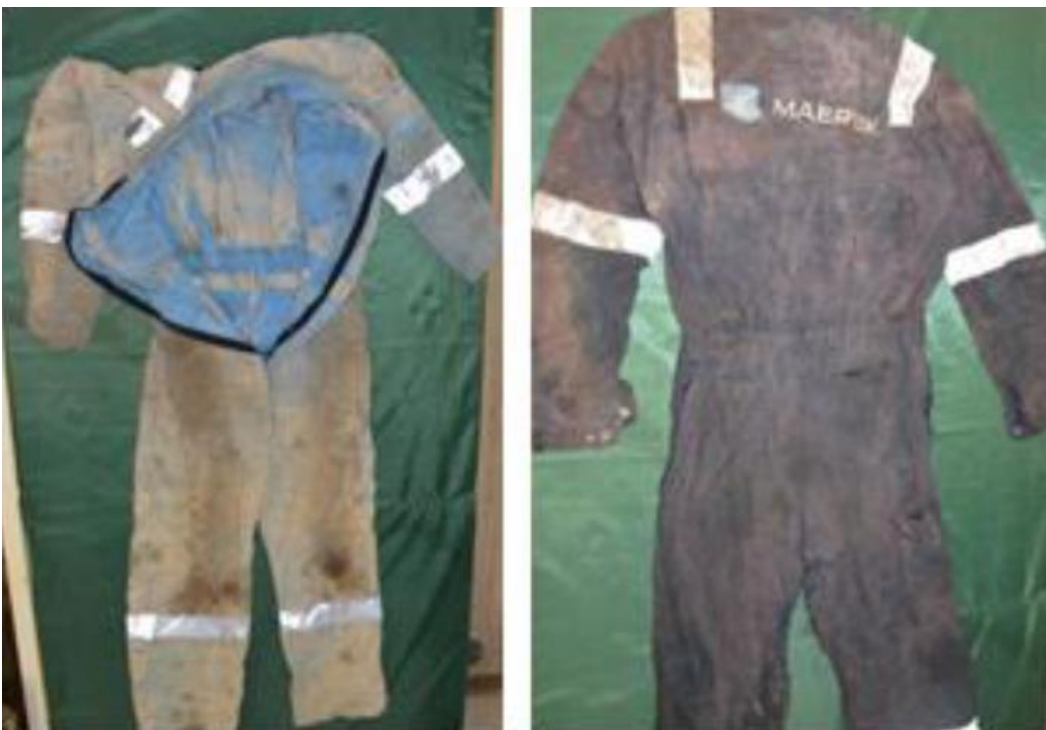
The formerly blue boiler suit on the left was bleached nearly white (Transport Safety Investigation Bureau)
